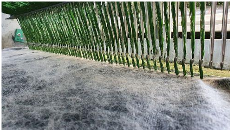
During operation of the tufting machine at the TFI, the needles pierce the carrier material (white) and thus insert the pile yarn for the artificial turf (green). Picture source: TFI
