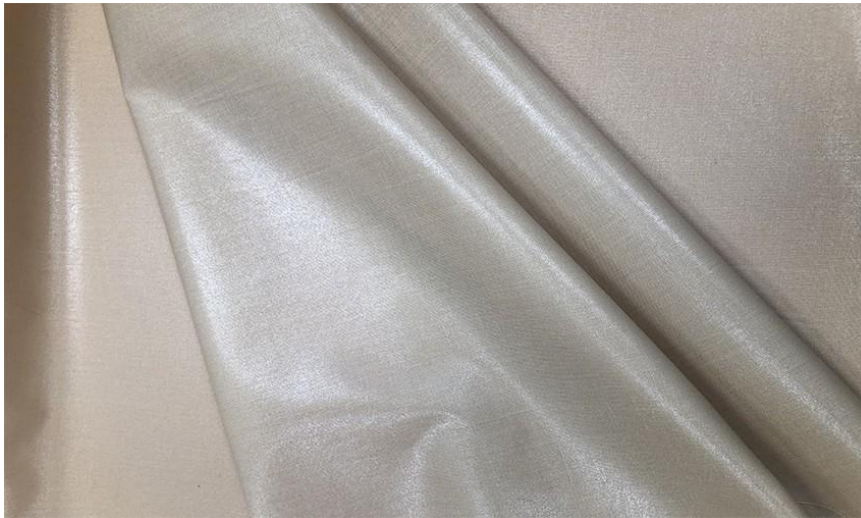
p-aramid fabric with silicone non-stick coating
