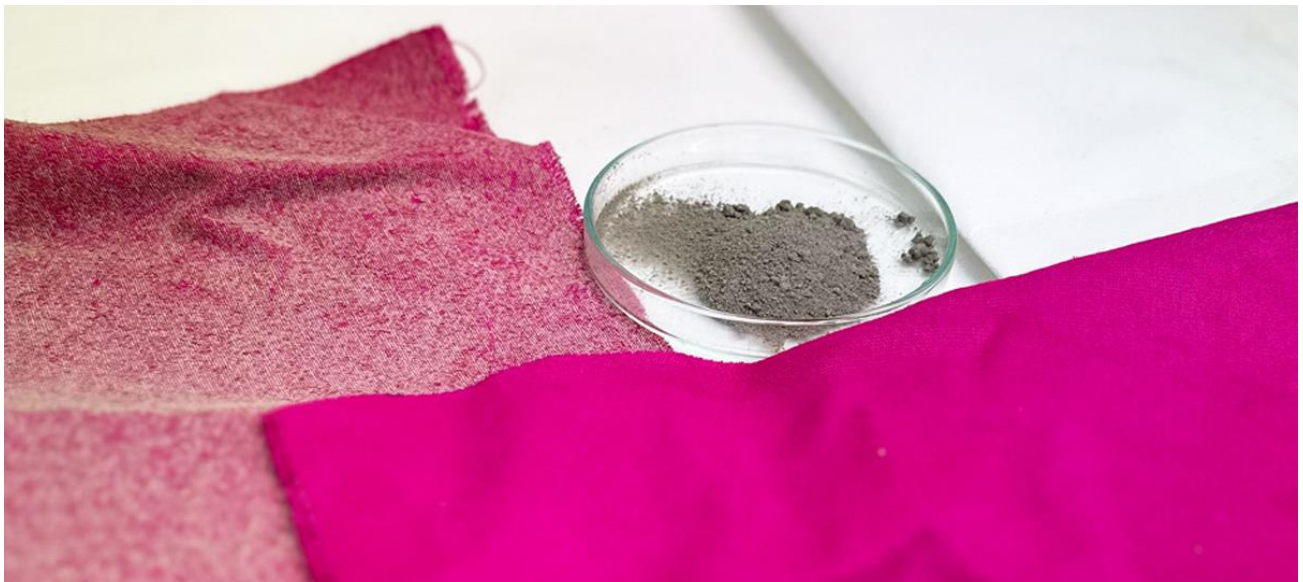
A sample of cotton that has been treated with nanodiamonds next to an untreated sample of cotton.
