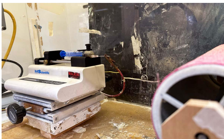
The electrospinning machine created a web of nanofibres on the cotton fibres, which are then cured to bond the two.
